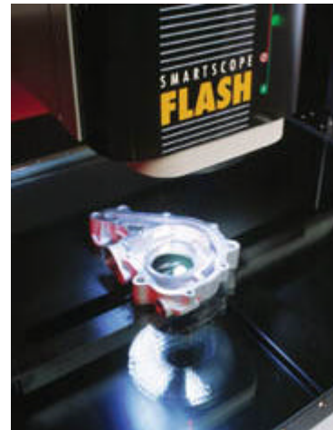
A video measurement of a cast metal part is illuminated by an LED ringlight. Photo: Optical Gaging Products
