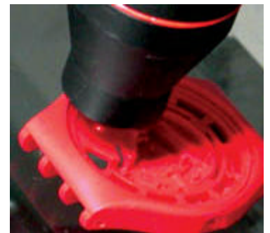
A spectral-analysis microprobe scans a small plastic part. Photo: Optical Gaging Products
