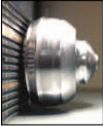
A close-up of the cone held on the magnetic fixture. The cone's entire profile and key features are measured in minutes.
