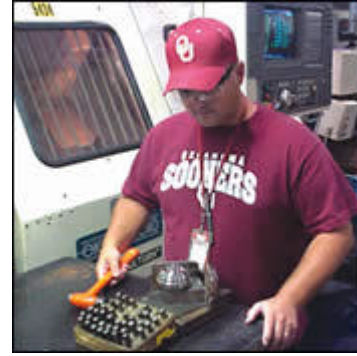
This CNC lathe operator is about to stamp a part number on this just-turned rock bit cone. Three meshing cones, each with slightly different geometry, go into each rock bit assembly.
