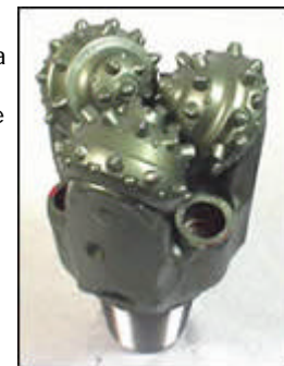
View of an assembled three-cone rock bit.
