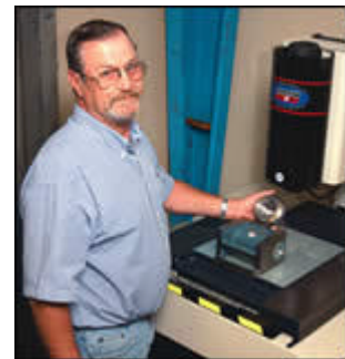
A machine operator loads a turned cone on a magnetic fixture positioned on the stage glass of this video-based measurement system, one of three such systems located in the machining area.
